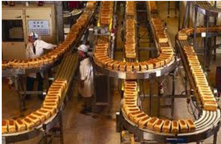
Figure 3. Industrial line for bread baked in tins production
