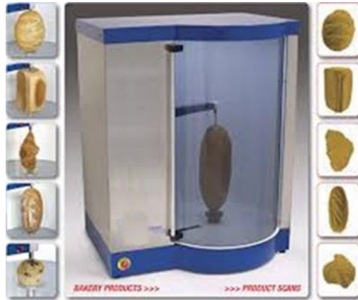
Figure 33. Loaf volume determination (source: www.stablemicrosystems.com )
