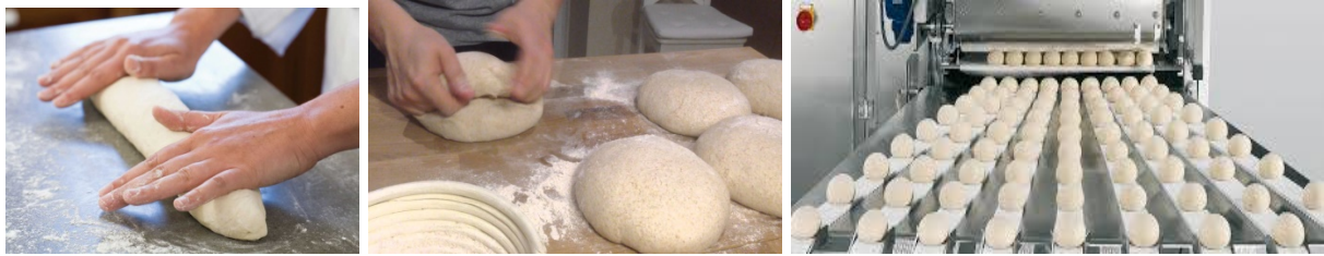
Figure 16. Different shaping operations performed on divided pieces of dough after bulk fermentation (source: internet)
