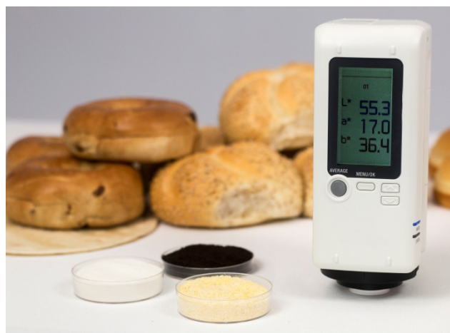
Figure 32. Rapid device for bakery products color determination
